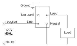
Figure 3: Connecting the switch
