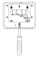
1. With a small phillips screwdriver, undo the locking screw from the back of the panel, remove the SmartMount backplate.
