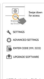
NOTE: For UL/cUL or EN Grade 2 installations the remote software feature shall not be used and the panel shall not be setup to remotely upgrade.
