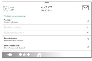
**NOTE**: 6 digit User Codes are required in order to Enable Control 4 integration.
