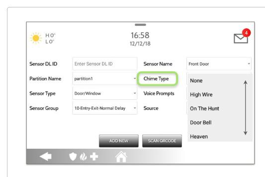
Because of the dynamic nature of the way the IQ Panel 4 pairs and understands each individual sensor, you can program each sensor to have a unique chime or even turn chiming off for that individual sensor. To customize your chime for a particular sensor touch the Chime Type drop down and choose from the list.
