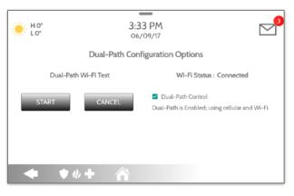
By default Dual-Path Control is enabled. To disable, "un-check" the box
