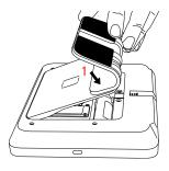
Locate the SmartMount table stand and insert the hooks into the back of the panel, then swing down and press into place.
