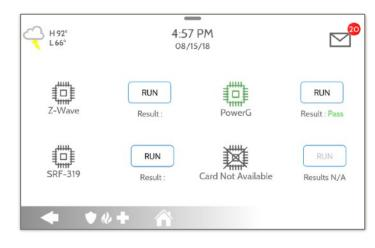
Select "Run" on an individual available card to start the test. In some cases the test may take several minutes after which the panel will show a result of a "Pass" or "Fail".
