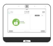
To access the Advanced Settings menu pull down the Settings tray at the top of the screen, select "Settings" and then "Advanced Settings". Enter your dealer, installer or master code. The code used to enter Advanced Settings determines the level of access. When using partitions the code entered at the screen lock determines the access level for Advanced Settings.
