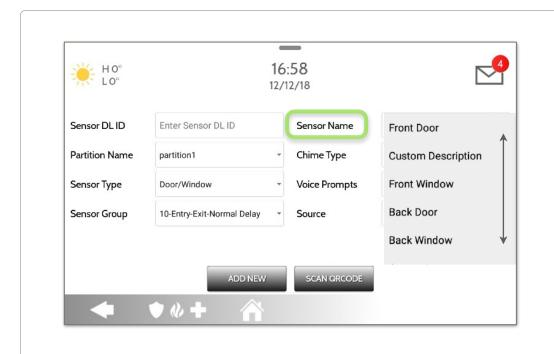
When you select the sensor name field you can choose from a variety of preset sensor names by scrolling up and down or create a custom description.
