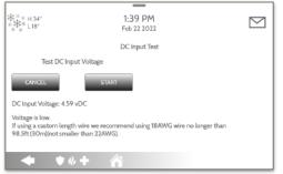
If voltage is below 6vDC, you will receive a "Voltage is Low" message and action should be taken to correct the low voltage condition (i.e. use thicker gauge wire or shorten the wire run).
