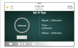
A successful test will result in a "pass" and indicates the date and time of the test along with connection speed.
