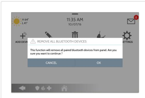
To delete and remove all enrolled Bluetooth devices at once, select "Remove All Devices".
