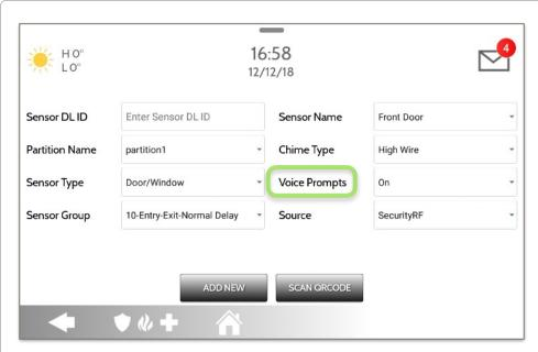
Voice prompts annunciate the sensor name when the sensor is opened or tripped.\*
