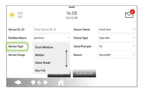
Note: for UL/cUL, only UL/cUL listed devices shall be used: Door/Window contact: 60-362N-10-319.5, Motion Detector: 60-639-95R, Smoke Detector: IQ Smoke QS5110-840. For UL2610 installations use only UL listed PowerG devices.
