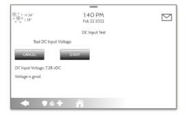
Press "Start" to run a real-time voltage test on the Panel. If voltage received is above 6vDC, you will get a "Voltage is Good" message.
