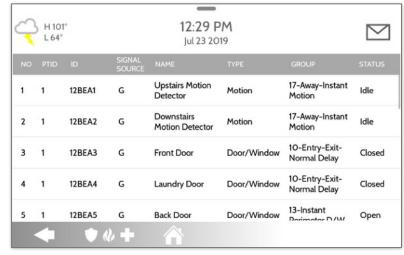
This page also allows you to quickly review programming for things like Zone number, Partition, Signal Source (319, 345, 433, PowerG, Native or Zigbee), Sensor Name, Sensor Type and Sensor Group.
