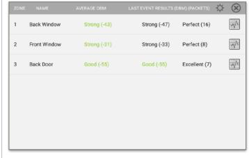
The Advanced Sensor Test shows a summary page of each sensor paired to the panel along with the average dBm level, the last event's dBm level and how many packets were received from the sensor.
