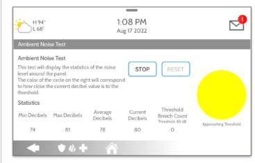
Select "Start" to perform a test of the Panel Ambient Noise Detector. You can Stop, Resume or Reset the test at anytime.
