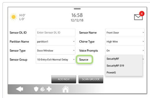
Source indicates the sensor's incoming frequency when pairing to the IQ Panel 4.
